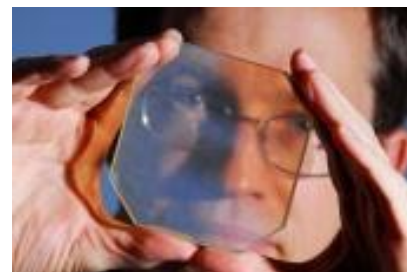
Figure 8: With Orlando-based OptiGrate, GTRI senior researcher David Roberts designed & fabricated a target board that can survive high-energy laser irradiation without changing its properties or significantly affecting the beam.
